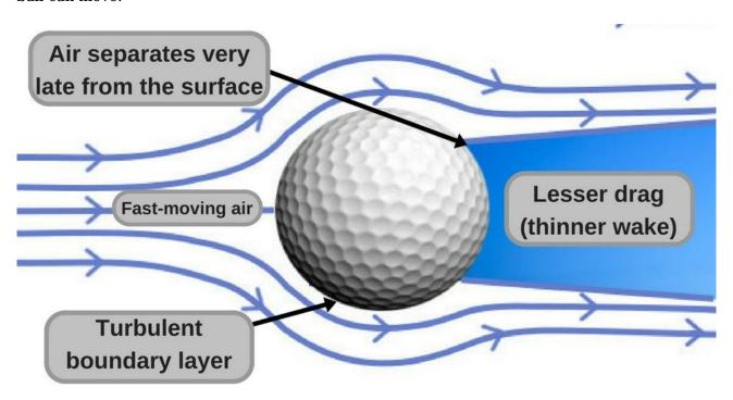
When air moves around any object, it exerts force. An object with an aerodynamic shape
